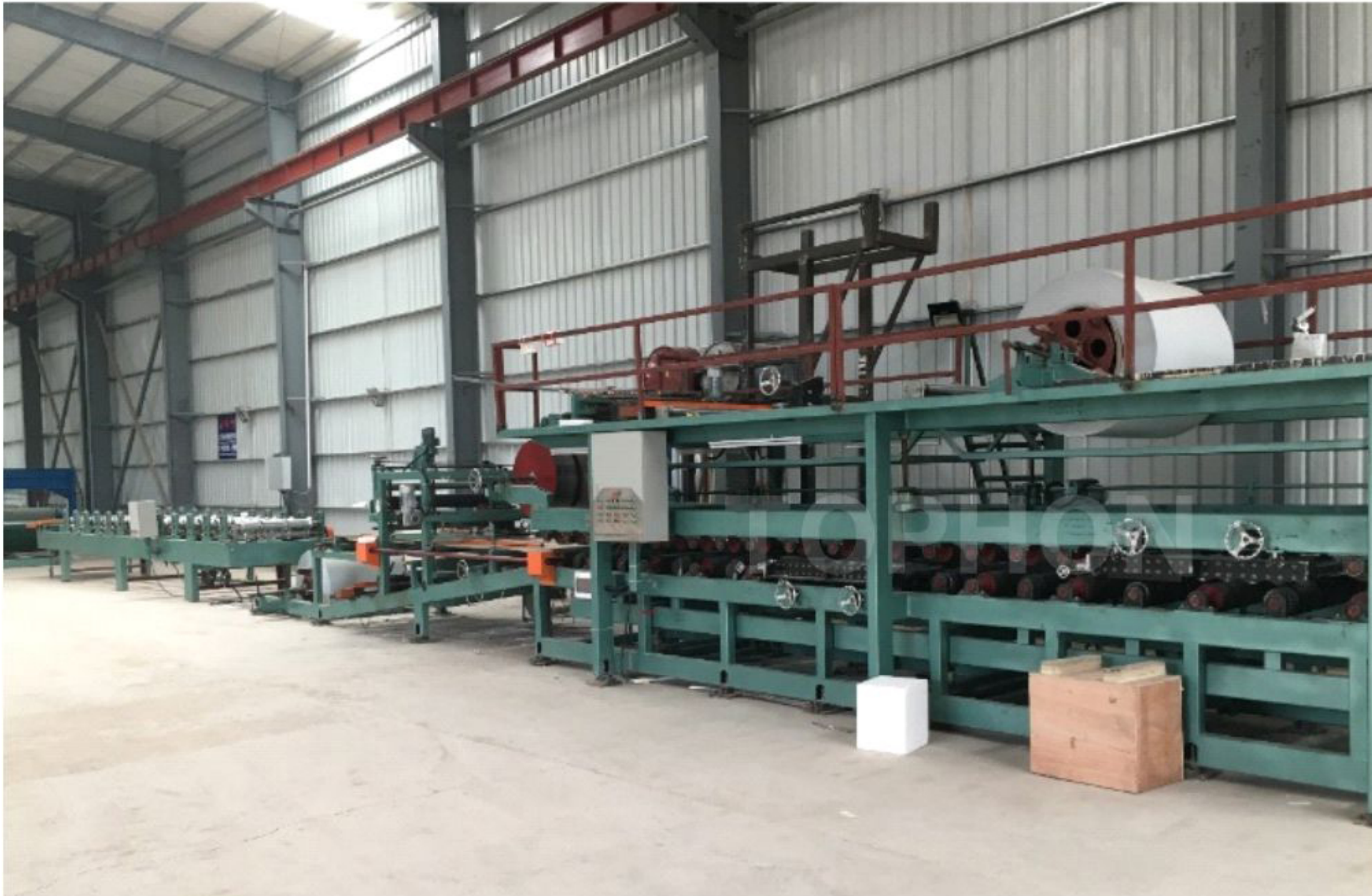
continuous EPS sandwich panel production line
